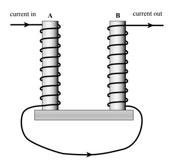
The electromagnet is powered by a **250 volt** power supply and is operated using a control unit. The resistance of the control unit is **1.8**  $\Omega$  and the combined resistance of both coils is **5.7**  $\Omega$ . The power supply, control unit and the coils of the electromagnet are connected in series, as shown in the diagram below.
